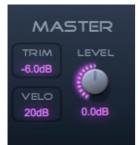
The master section controls the output level. The TRIM parameter controls the the current preset's output level and the VELO parameter controls the velocity sensitivity of the current preset's output level. The TRIM and VELO parameters are recalled for each preset. The LEVEL parameter controls the plugin's output level regardless of the current preset.
