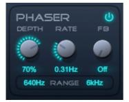
The phaser effect's sweep is controlled by the modulation rate and frequency range. The DEPTH parameter controls the intensity of the phaser. The additional intensity i.e. the amount of feedback is controlled by the FB parameter.
