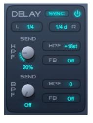
The delay section runs two delay units in parallel, a high pass filter delay and a bandpass filter delay. The high pass filter precedes the delay unit in the signal chain of the high pass delay whereas the bandpass filter follows the delay unit within the feedback chain of the bandpass delay.
