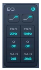
The equalizer section has two units. The mode can be selected from the list independently for both units. The Q and GAIN parameters have effect only in certain modes.
