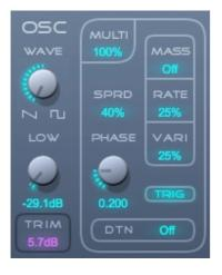
Oscillator section controls the shape of the waveform used in Kairatune's tone generator. The shape of the waveform can be tweaked from simple sawtooth or square wave, known from classical analog synthesizers, to complex and vivid multi oscillator waveforms.
